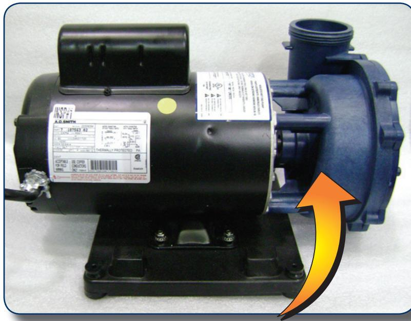
Blue wet ends are an industry standard to ensure that the pumps were manufactured for hot water and are not pool pumps.
